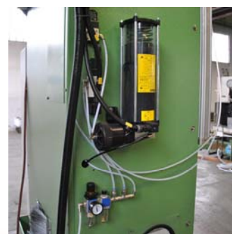
Timed pump for grease distribution
