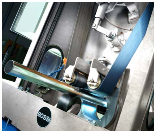
Detail of the abrasive belt working on tube external weld bead
