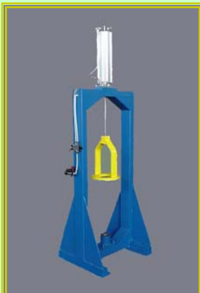
Press for assembling the polishing mops, with pneumatic control
