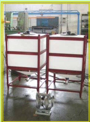
Storage bins for liquid abrasive compound
